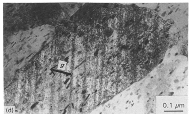
Figure 9 Comparison of the distribution of slip bands after 1% tensile strain: (a) Alloy 1, B = [01\bar{3}] , g = [200] , (b) Alloy 2, B = [011] , g = [02\bar{2}] , (c) Alloy 3, B = [011] , g = [02\bar{2}] , (d) Alloy 4, B = [\bar{1}12] , g = [220] .
